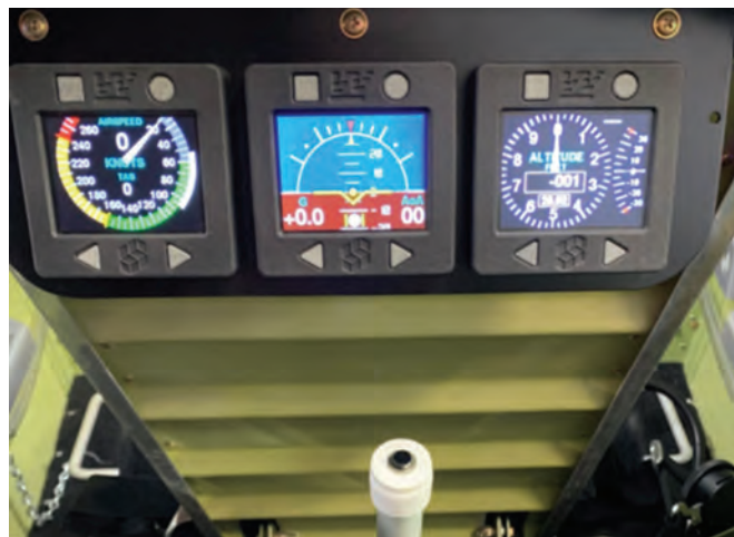
▲ The huVVer-AVI programmable electronic flight instruments, distributed by MakerPlane in Gatineau, configured as a back-seat panel in a Harmon Rocket.
