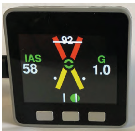
▲ An OnSpeed energy display prototype. The white horizontal bar lines up with the two white dots to indicate the best lift-over-drag ratio, corresponding to best glide and best rate of climb angle of attack. A green dot in the centre lights up to indicate the best approach and best climb angle of attack, aka ONSPEED. The red chevrons indicate low energy and flash to indicate approaching stall.
