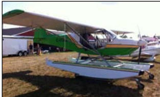
2011 RANS S7S ON ZENAIR 1450 AMPHIBS. 213 TTSN. Rotax 100hp. Electric flaps, Elis, twin radio, iPad mini dash mount, Transponder. Much more options. 200 hour just done by Rotax. $89,000. fwleslie@eastlink.ca. NS, Canada. (2951.16084)
