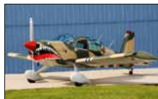
GRUMMAN TAIL DRAGGER $29,900 CDN for 50% share in this rare Grumman AA1B tail wheel conversion Last of 30. NDH 150HP O320 138 KT cruise. 7.1 GPH 1,300 FPM climb! 2435 TTAF 237 TTE&P. 74DM6 prop Mattison tip mods Aux fuel w/32G useable Skytech lightweight starter STC'd Oil cooler. EI Fuel computer. New EI EGT, Wing leveller, NEW Bendix King Radio King Mode C CHT Vert od compass Carbon fibre spinner and wing tips. Red rudder cap. New tires/tubes/Gill battery. Panel mounted GPS. NEW CARB. Heated Hangar. Contact: 5192727135 or jason@mccannrealtor.ca (3126.17338)
