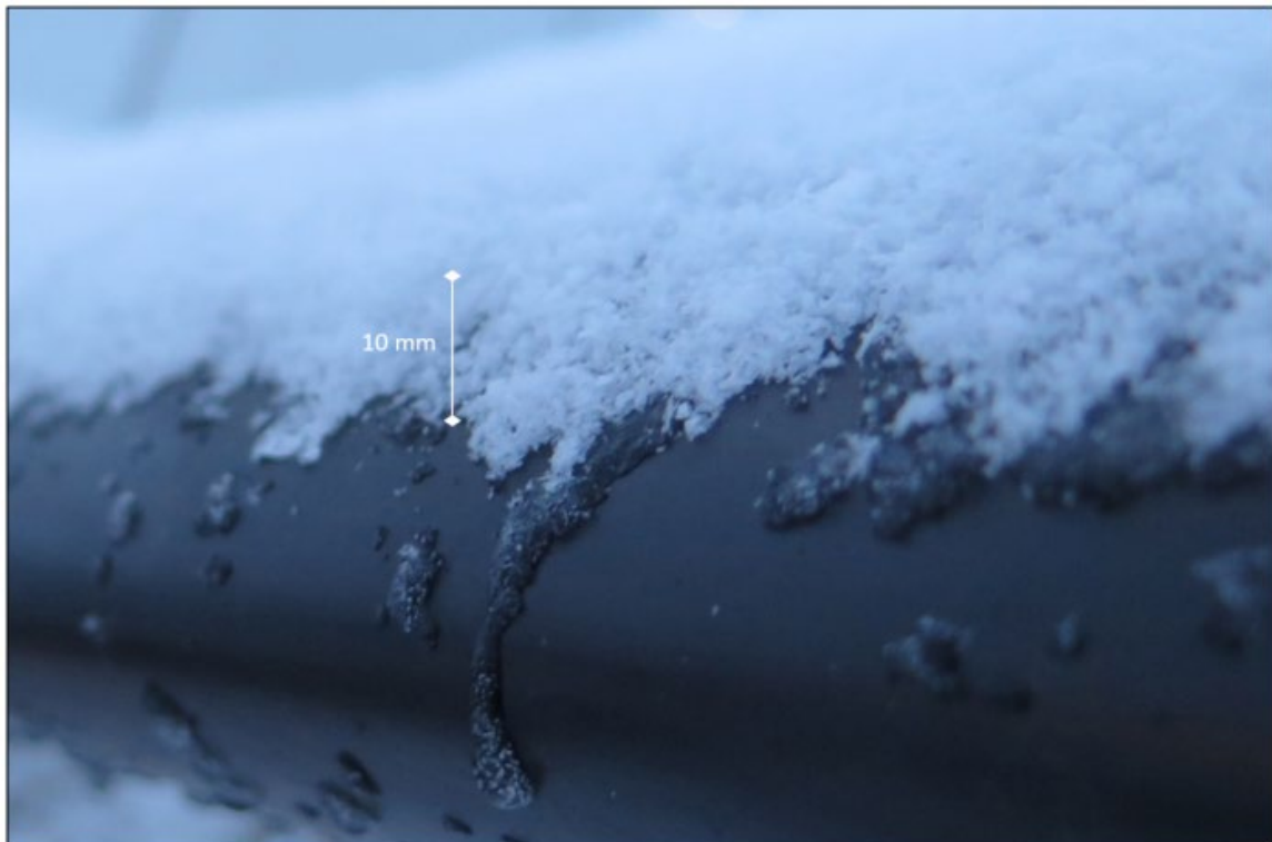
Figure D4. Occurrence wreckage demonstrating the melt/refreeze process approximately 8 hours after the occurrence
