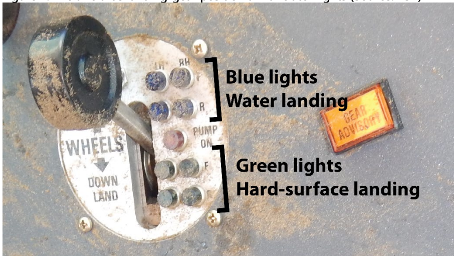
Figure 2. The aircraft's landing-gear position annunciator lights (Source: TSB)
