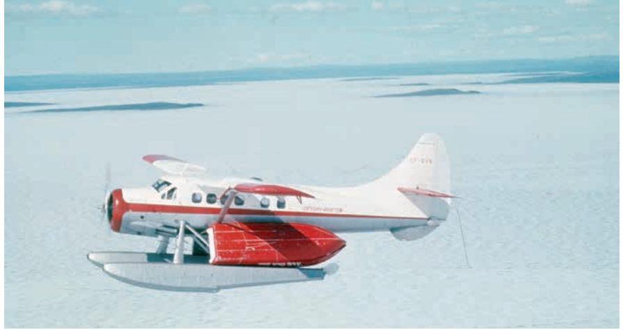
▲ Flying in July across Great Bear Lake with two aluminum boats for American sports fishermen at Arctic Circle Lodge. During this flight, the Otter was barely maintaining altitude at climbing power.
