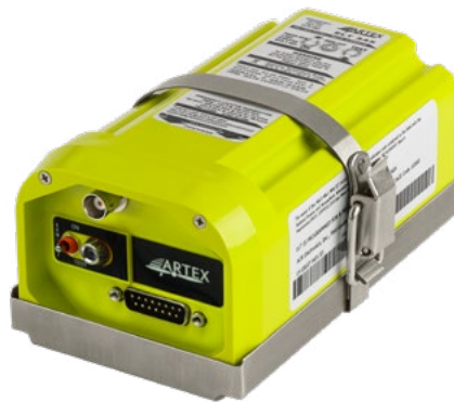
▲ The Artex ELT 345 transmits on 406 MHz and 121.5 MHz.
