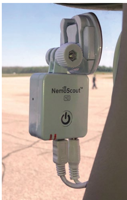
▲ The NemoScout aircraft to aircraft radio data network extends the tracking coverage of each equipped aircraft.
