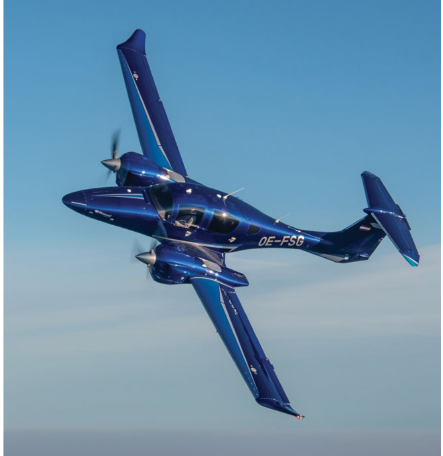
▲ Leveraging a six-cylinder, 300-horsepower Continental CD-300 diesel engine, the DA50 RG is rated for a max speed of 181 KTAS and 20,000-foot ceiling.
