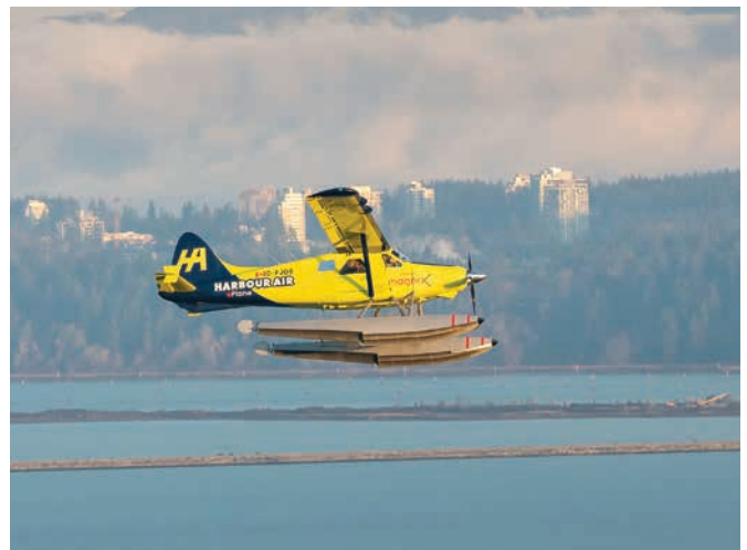
▲ The Harbour Air ePlane in late-2019 takes its first flight over the Fraser River in Richmond, BC; powered by the magniX magni500, a 750-horsepower electric propulsion system.
