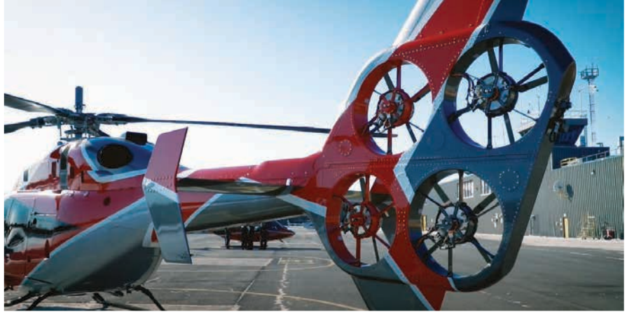
▲ Featured on a 429 testbed, Bell’s Electrically Distributed Anti-Torque system is composed of four small fans within a tail rotor shroud in an offset two-by-two pattern.
