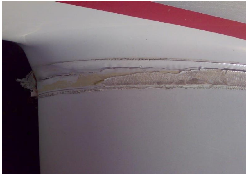
Damage to Diamond Katana wing root caused by sun exposure
