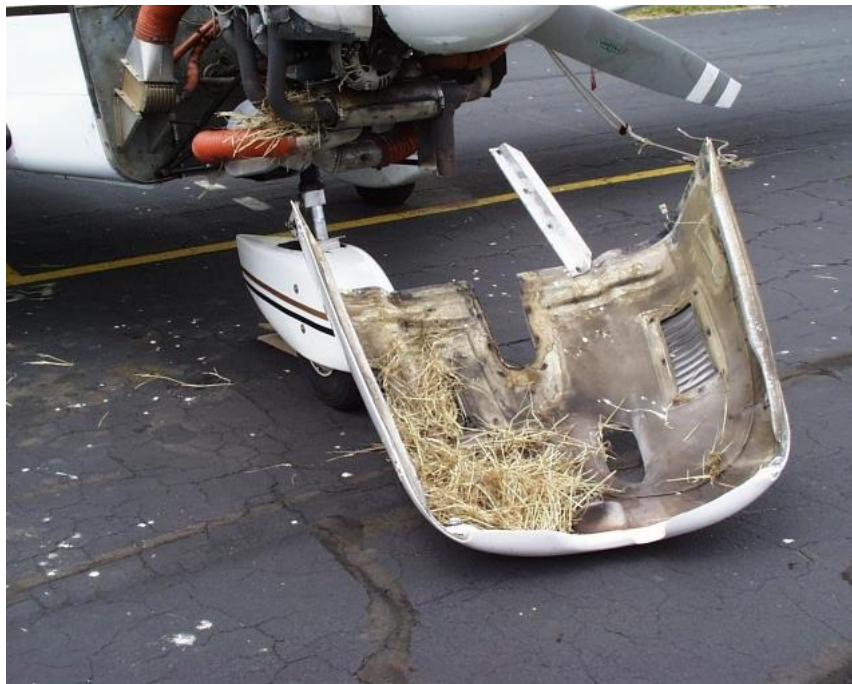
Photo from Aircraft Owner's and Pilot's Association (AOPA) of a bird's nest built in a cowling
